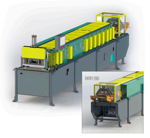
Jobsite manufactures the PS1200 in-plant machine for roll forming steel studs and track used in floor, wall, and truss framing. This machine can form studs or track from 8" to 12" with 26 to 14 gauge steel.
